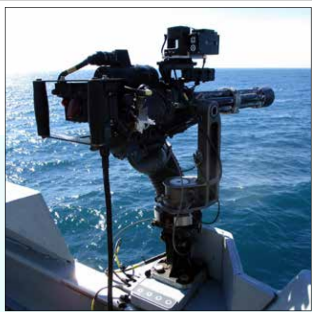
● A minigun equipped with the Pointer T targeting system fitted to a Type 23 frigate
