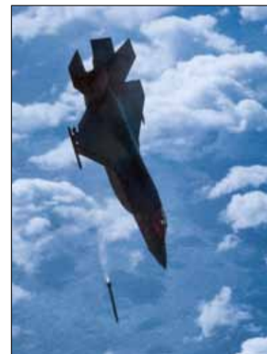
● Above, a Paveway IV bomb is dropped by an F-35; right, the test firing of ASRAAM from BF-03
