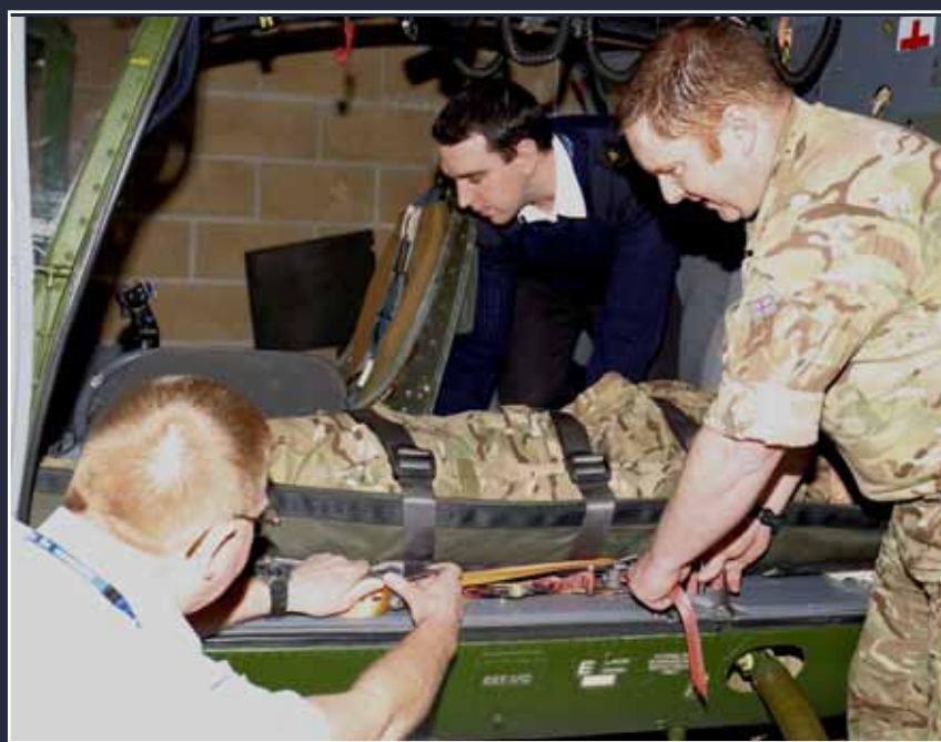
● The 1710 NAS team show how a stretcher with a casualty can be placed inside the adapted Gazelle helicopter
