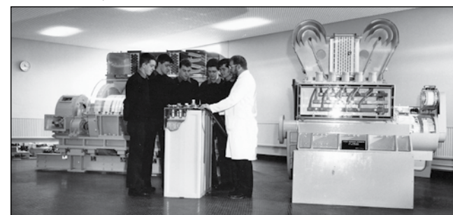
● Students at HMS Sultan examine a submarine battery cell, possibly in the 1970s; the machine to the right is a 1,000kw brushless alternator, while behind them is a motor generator
