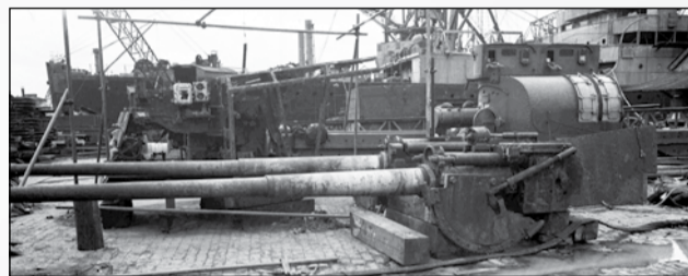
● The 10.5cm flak guns as they appeared mounted on the wreck of the Graf Spee as photographed by British 'salvage' experts and (right) the only known images of the barrels and their mountings, taken for reasons unknown in Devonport in July 1942
